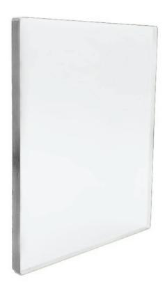
Phillips Lead Acrylic Windows combines reliable radiation shielding with exceptional clarity, making it one of the clearest options on the market. With an impressive 87% visual light transmission, these windows provide unobstructed views while maintaining robust protection. Their thickness of 12±0.7 mm offers a lead equivalency of 0.50mm Pb Eq, ensuring they meet stringent safety requirements.
