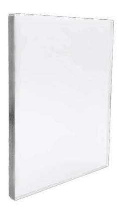
Phillips Lead Acrylic Windows .33mm pb combines reliable radiation shielding with exceptional clarity, making it one of the clearest options on the market. With an impressive 90% visual light transmission, these windows provide a clear view while offering radiation protection. Their thickness of 8±0.5 mm offers a lead equivalency of 0.33mm Pb Eq, ensuring they meet stringent safety requirements.
