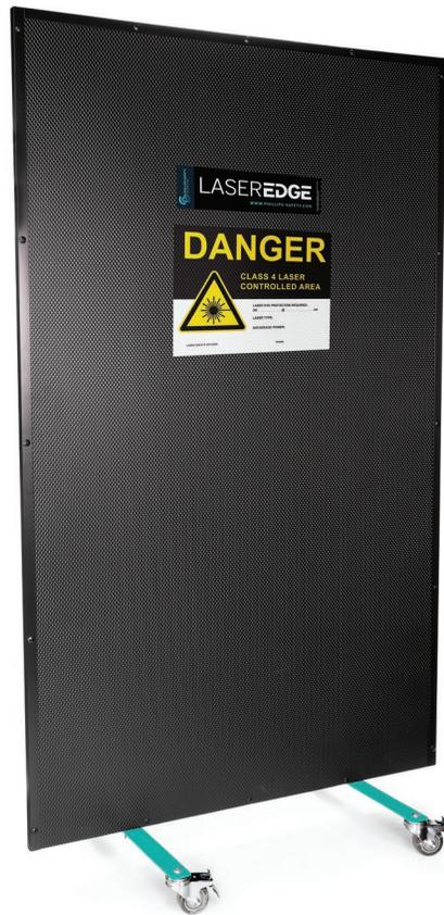
The LaserEdge Rigid Laser Safety Barrier is designed to withstand a laser rated at 30 kW/cm<sup>2</sup> for 100 seconds. Constructed with a lightweight aluminum frame, it features cross braces, locking wheels, and a freestanding design. Available in a standard size of 4ft x 8ft, it provides reliable protection for a wide range of laser environments. Additionally, the LaserEdge Rigid Laser Safety Barrier complies with ANSI Z136 safety standards, ensuring top-notch safety in laser applications.
