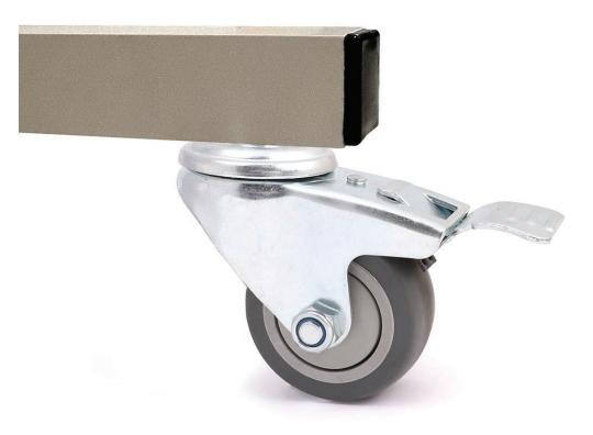
The Replacement Caster for Mobile Radiation Barriers is a locking caster with brake for mobile barriers. It has 75mm (3 in) wheel diameter, with a load capacity of 100kg. Please note that if all casters need to be replaced, you must select a quantity of 4 replacement casters.
