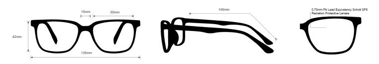
The radiation glasses Nike 8214 feature high quality, distortion-free SF-6 Schott glass radiation-reducing lenses with 0.75mm Pb lead equivalency protection. The radiation safety glasses Nike 8214 have clear CE Certified Lens and weight 88g. These radiation glasses Nike 8214 are prescription available. Made of high-quality metal, it is a durable and lightweight square frame for women. These Nike lead glasses feature adjustable silicone nosepads and are available in four colors.
