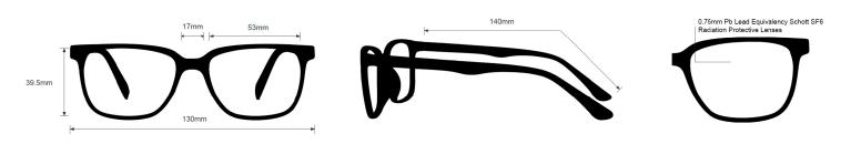
The radiation glasses Nike 7177 feature high quality, distortion-free SF-6 Schott glass radiation-reducing lenses with 0.75mm Pb lead equivalency protection. The radiation safety glasses Nike 7177 have clear CE Certified Lens and weigh 70g. These radiation glasses Nike 7177 are prescription available. Made of high-quality plastic, it is a durable and lightweight rectangular frame for women. Plus, these Nike lead glasses feature a saddle bridge and are available in four gradient colors.
