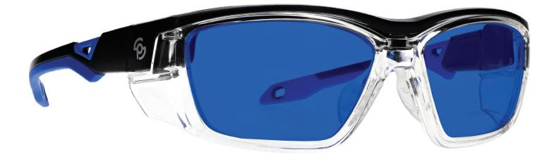
The lampworking glasses BoroTruView 2.0 have a polycarbonate royal blue glassworking lens that provides excellent color recognition for borosilicate glass and furnace work. These flameworking glasses offer excellent UV blocker, excellent IR protection, excellent sodium flare blocker, and excellent clarity. Recommended for those who work with lampwork or hot glass in small pieces.
