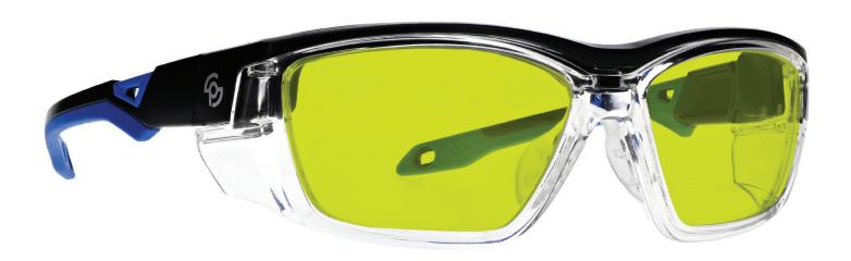
The glass blowing glasses Light Green have a polycarbonate light green lens that provides good color recognition for furnace work. These glasses for glass blowing offer excellent UV blocker, excellent IR protection, and good clarity. Recommended for those who work with glass blowing or any hot glass in small/large pieces.
