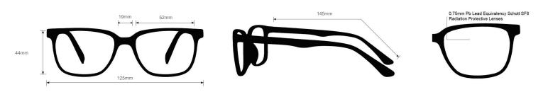
The Ray Ban radiation glasses Elliot feature high-quality, distortion-free SF-6 Schott glass radiation-reducing lenses with 0.75mm Pb lead equivalency protection. These Ray Ban lead glasses have clear CE Certified Lens and weigh 72g. Plus, the Elliot radiation glasses are prescription available. Made of high-quality plastic, they have a durable and lightweight square frame. These lead glasses feature a high bridge fit and are available in two color variations: polished havana and polished black.
