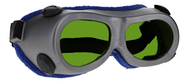
The YAGEXT laser safety glasses have a polycarbonate green lens filter that provides laser protection. These laser glasses have visible light transmission of 11%. Plus, the YAGEXT laser safety glasses meet ANSI Z87.1 and ANSI Z136.1 safety standards. Moreover, these laser safety goggles 55 have a durable and lightweight fitover goggles frame. Made of high-quality plastic, the 55 laser safety goggles feature strap. In addition, these Phillips Safety laser safety goggles are available in silver.
