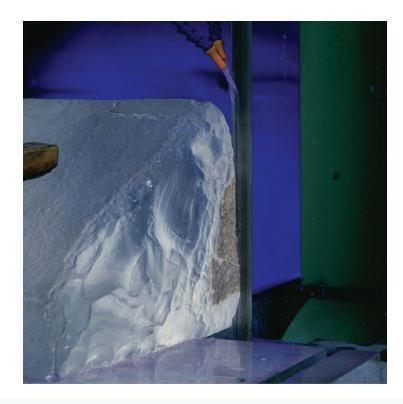
Fused quartz is a glass that can tolerate extreme temperature ranges and provide thermal shock resistance. It differs from other glasses in the fact that no additional ingredients are required to lower the melt temperature, giving it much higher working and melting temperatures.
