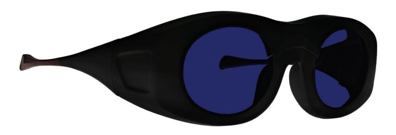
The Cobalt Blue welding fitover glasses 9014 have a glass cobalt blue welding filter shade 4.0, 5.0, 6.0, and 8.0, which provides torching and brazing protection. These Cobalt Blue torching glasses are ANSI Z87.1, EN 166 and EN 169 approved, and have CE certified lens.
