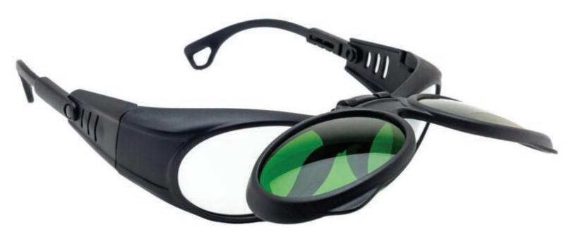
The Green welding glasses 17004 have a clear lens with polycarbonate green welding filter shade 2.0, 3.0, 4.0, 5.0, 6.0, 7.0, 8.0 in the flip-up, which provides torching and brazing protection. These Green torching glasses are ANSI Z87.1, EN 166 and EN 169 approved, and have CE certified lens.
