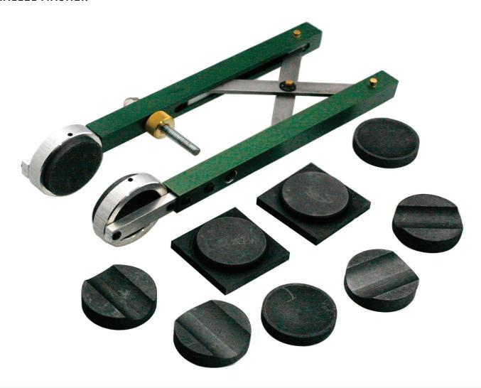
The Parallel Masher is a versatile tool designed for flattening and shaping glass. Made of high-quality aluminum, this masher comes with a set of two graphite round flat heads measuring 1.75" in diameter. Other head shapes are also available separately, including a lentil head, a small radial head, a large radial head, and a 2" square flat head. For more information about different replacement heads, check out our Mashers collection.
