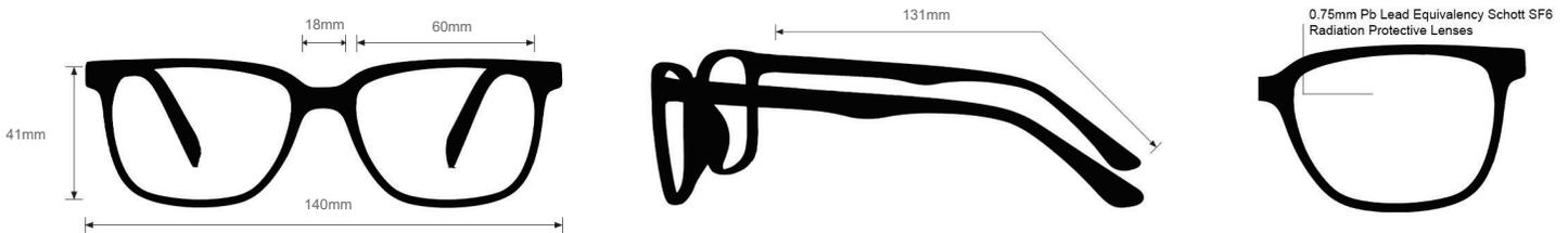
The radiation glasses 39 feature high quality, distortion-free SF-6 Schott glass radiation-reducing lenses with 0.75mm Pb lead equivalency protection. The 39 lead glasses have clear CE Certified Lens and weight 87g. These radiation glasses 39 are prescription available. Made of high-quality plastic, it is a durable and lightweight wrap around frame. These Phillips Safety prescription radiation glasses are available in black.
