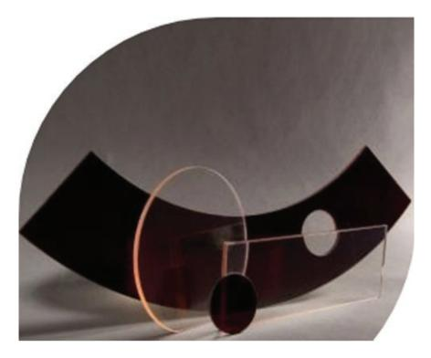
Glass ceramic is often recommended for applications that require extreme heat capabilities and UV blocking traits as well as virtually zero thermal expansion. Due to its extremely low thermal expansion, it can be subjected to extreme temperature differences. In high temperature conditions, it retains excellent form stability. Glass ceramic can be further developed with all of the normal methods of glass processing.
